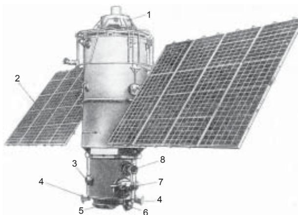
Fig. 5 First-generation Meteor (Kosmos-144). Key: 1. solar panel orientation system, 2. solar panel, 3. orbit control equipment, 4. antennas, 5. MR-600 television camera, 6. magnetic sensor, 7. receiver of actinometric equipment, 8. Lastochka infrared radiometer. (source: Mir Publishers)
