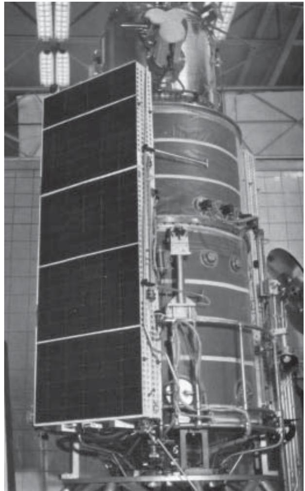
Fig. 9 Meteor satellite in final assembly.
