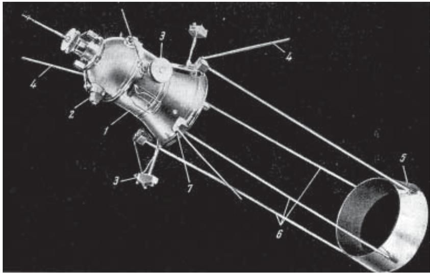
Fig. 2 The DS-MO satellite. Key: 1. satellite body, 2. television equipment, 3. sensors, 4. antennas, 5. aerodynamic stabiliser, 6. boom, 7. boom deployment mechanism. (source: Nauka publishers)
