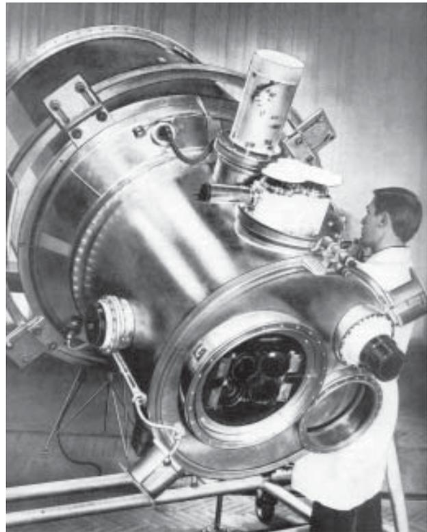
Fig. 8 Meteor payload compartment undergoing testing. (source: Gidrometeoizdat)
