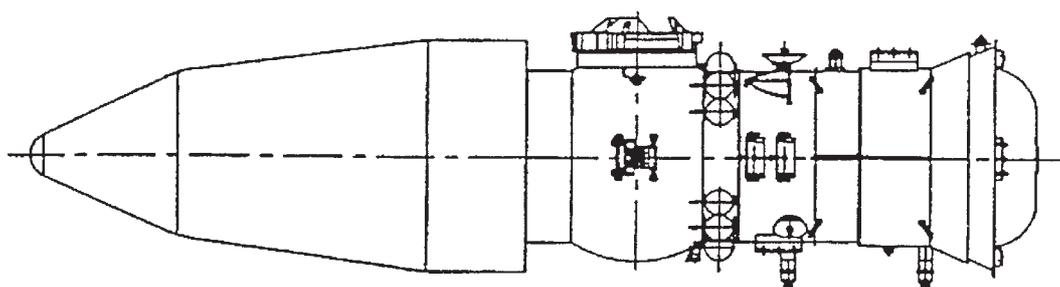
Zenit-launched manned spacecraft with lifting body re-entry vehicle proposed in the early 1990s.
