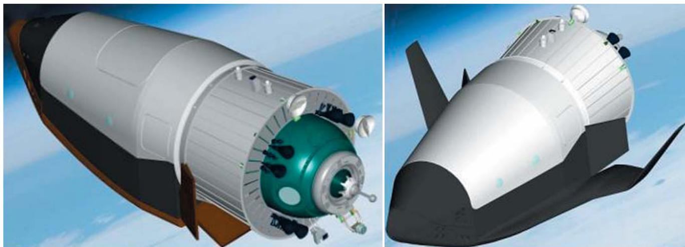
Two currently proposed versions of Kliper: a lifting body and a winged vehicle.
