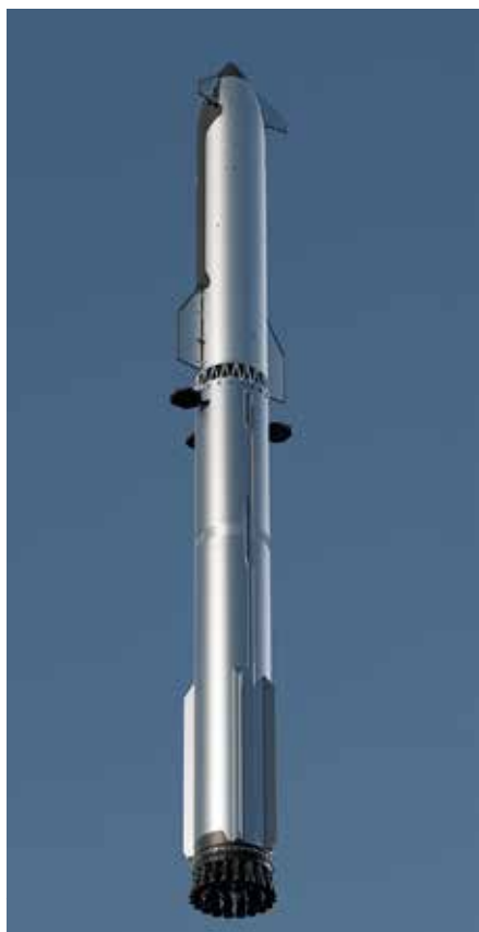
SpaceX's Starship version three's key external design differences can be seen in this official illustration showing the exposed Raptor engines, the three, instead of four, grid fins on the first stage Super Heavy booster, and the fixed hot staging adaptor.
